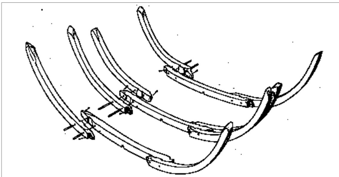
Fig. 5. In this drawing, the same three floor timbers are shown with their futtocks, illustrating the dovetail mortise assembly. Robert Hellier, Parks Canada.
